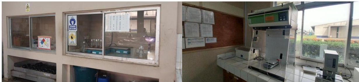
Plate 2.10: Static and Mobile Fume Cupboard
